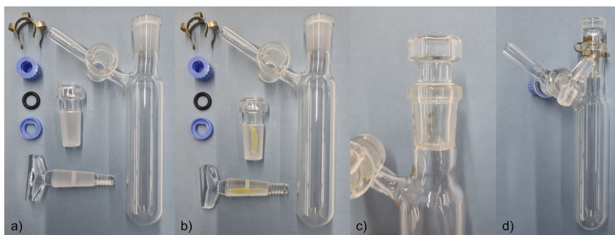
Figure 2. Greasing and inserting a ground glass stopcock and stopper into a Schlenk flask. A hydrocarbon-based grease is shown for clarity.
