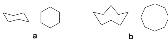
Fig. 48 Side-on perspective view ( left ) and view from the top ( right ) of a chair of cyclohexane, and b crown of cyclooctane
